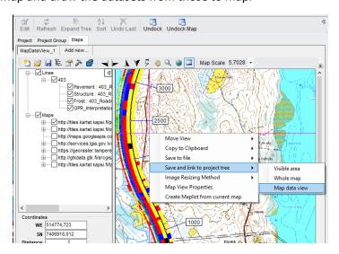
As a new feature it is also possible to **update the thematic map in a Map View** if the source data in a view is changed. This makes possible to keep the analysis fields in the map and in the view synchronized. Also, if a database content is modified, the modifications for a displayed field can be updated to a map.
