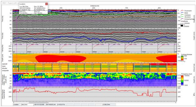
• Different modules for deeper analysis of Road Data using Frequency and bearing capacity analysis methods.
