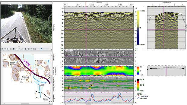
New **user defined colour tables** can be defined for GPR data display. The maximum number of colours is 256. The table with less colours (128, 64, 32, 16) can be created automatically. The new colour table is saved in the view and can be used later.
