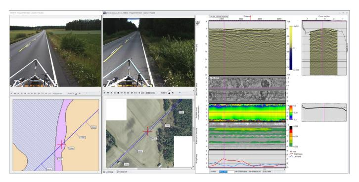
Advanced tools for GPR data processing and interpretation and comparing GPR data with other data from different measuring devices like Video, LIDAR, FWD, Profilometer, TSD, etc. and from local or external databases or any WMS- and Google maps.
